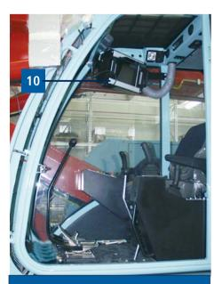
New cab w. Drilling Mate System
